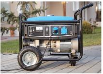
A portable generator is usually gas-powered and movable. A generator should have more output than the wattage of the electronics plugged into it. This way, the generator will be able to create the extra electricity it takes for the initial power surge. Make sure there is nothing plugged into the generator when turning it on.
